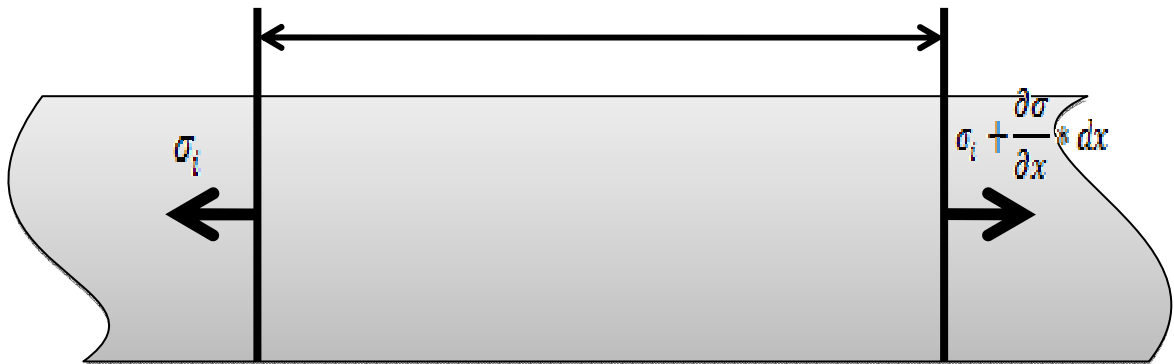
Figure 2.4- Constrained Rod with a Longitudinal Stress Wave
